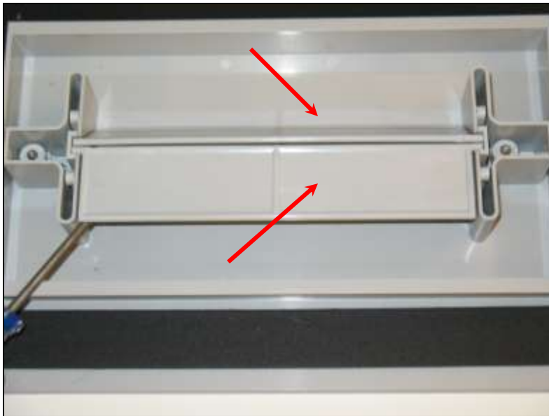
Inlet flaps, check for free movement.
