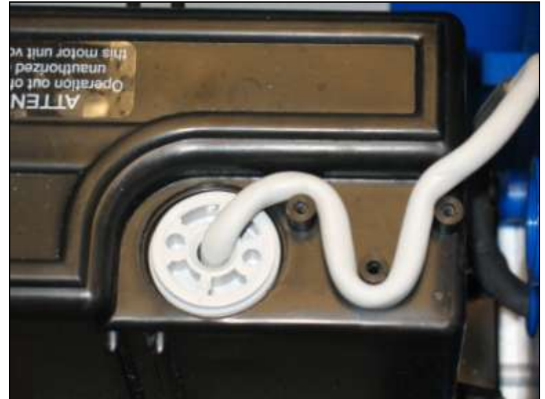
Plate removed showing strain relief system.
