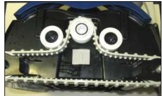
Drive side view with cover removed.
