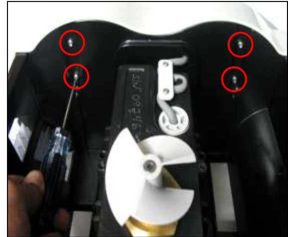
4 T20 screws each side to remove for side plate removal.
