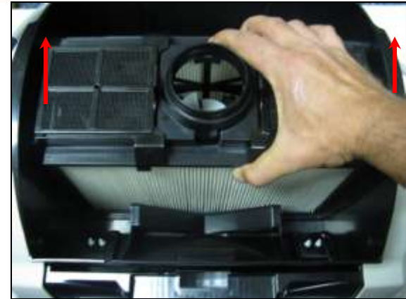
Lift to remove Filter Bucket Housing
