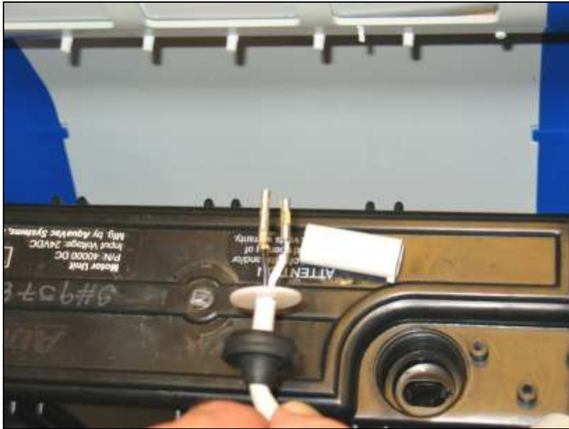
Power cord electrical pins removed from connector. Note that white wire goes on tab side of connector.
