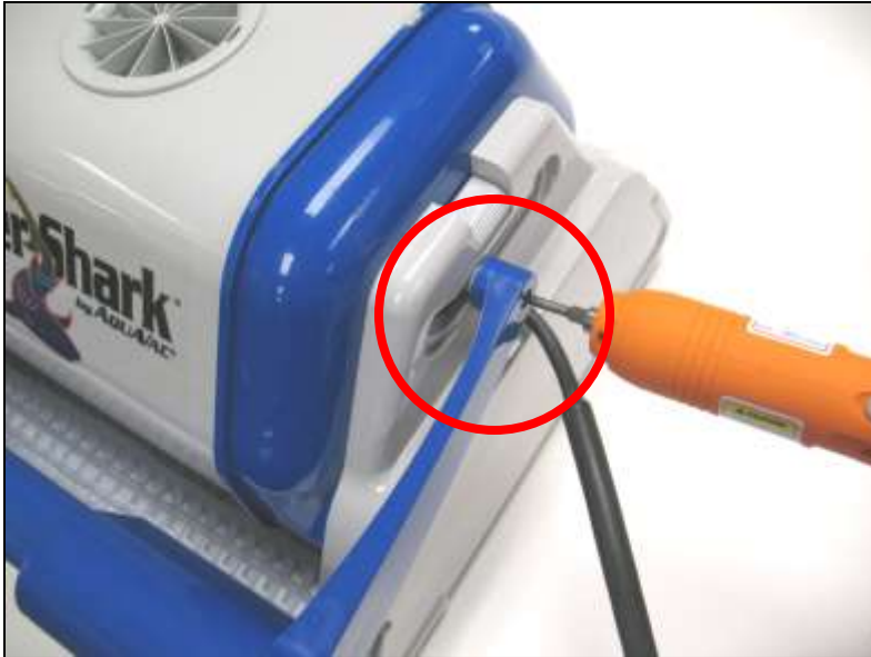
Handle removal 1 screw each end
