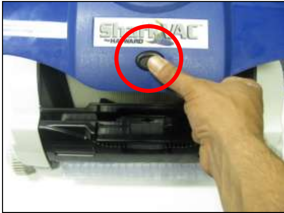
Press Dome Button to lift Dome for filter removal.
