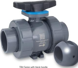
TBH Series with black handle identifier, drilled ball for sodium hypochlorite applications.
