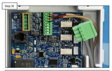
Remove the RS485 Communication block. IF the Wiring Hub Comm Error clears, something in the block is causing the problem (i.e. VSP or Smart Relay). IF problem persists, replace the Controller (HLHCONTROL)
