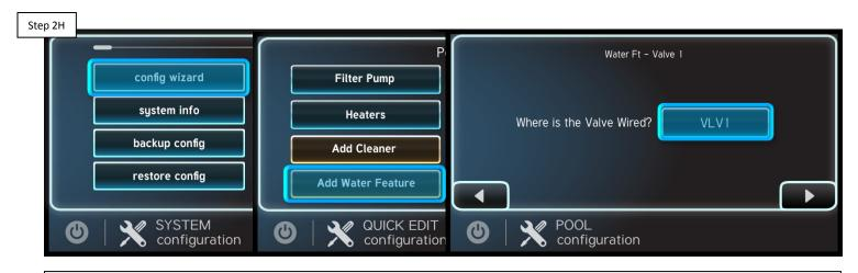
Using quick edit, reprogram the valve. IF the valve still will not rotate while being activating through the controller, then please contact support (908) 355-7995 for additional support.
