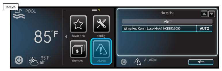
On the display, select the "alarm" icon (on right side of the screen). IF an Comm Loss – Wiring Hub appears go to section 3, IF it does not appear, go to 2B.
