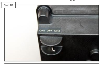
Locate toggle switch (bottom of actuator). Verify switch is either in ON1 or ON2 positions. Toggle the switch between ON1/ON2, IF actuator does not move, go to step 2E, otherwise skip to step 2G.
