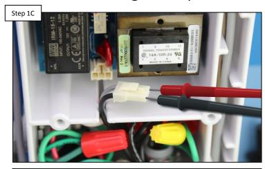
Unplug input power connector. Verify 120 or 240vAC. IF 120/240vAC is present, replace the hub PCB (HLXHIOPCB). IF not, go to step 1D.
