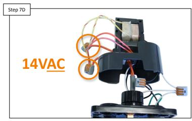
Open lighting transformer and test for 14vAC on the output side. IF voltage is correct on the output side of the transformer, replace defective lights. IF no/low voltage, go to step 7E.
