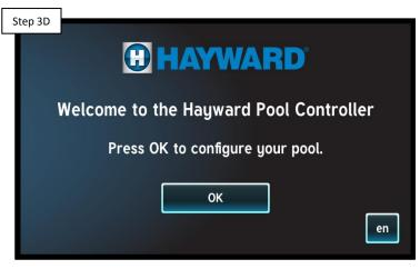
Reset the system to factory default and reprogram. IF the Wiring Hub Comm Error clears, then back up the configuration. IF problem persists, go to step 3E.
