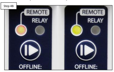
Inspect the two LED indicators on the front of the Smart Relay. There is a Remote LED and a Relay status LED. IF no LEDs appear, go to Step 4C. IF any LEDs are lit/flashing, jump to Step 4D.
