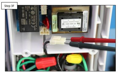
Unplug input power connector. Verify 120/240vAC. IF 120/240vAC is present, replace the hub PCB (HLXHIOPCB). IF no/low, resolve at the breaker/timeclock.
