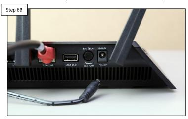
Power cycle the network router and confirm the 2.4Ghz Wi-Fi signal and password. Retry network setup under: config>network. After running network diagnostics: IF no red flags were generated AND the problem persists, please contact support (908) 355-7995\*. IF red flags appeared, proceed to Step 6C.
