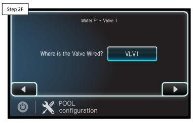
Reprogram the value using quick edit. IF the valve still does not rotate when turned ON through the controller, replace the Hub PCB (HLXHIOPCB).
