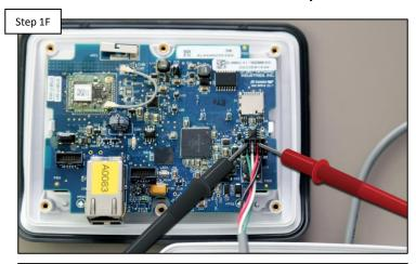
Test cable that plugs into controller PCB for 12v<u>DC</u> between terminals 1 & 3 (left to right). IF power is present, replace controller (HLHCONTROL). IF no/low voltage replace controller cable (HLX485100).
