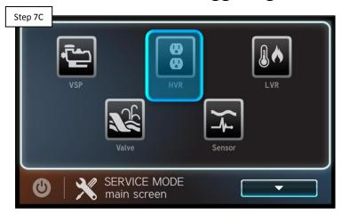
Put system in service mode (power>service mode), then toggle lights on, off, & back on. IF lights are illuminating, install a snubber & resync lights after exiting service. IF they did not illuminate, go to 7D.
