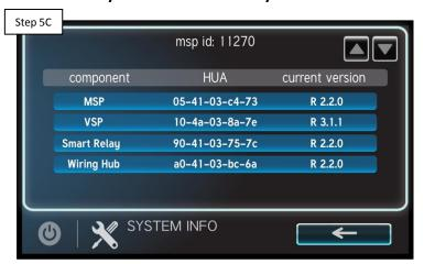
Navigate to Config>System Info and verify the Pump HUA is showing up in the list. IF HUA does not appear, go to 5D. IF it does, reprogram VS Omni, contact support if the problem still persists: (908) 355-7995.
