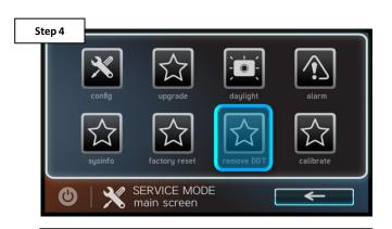
Select "remove DDT", then check mark. After system is wiped clean, then power cycle.
