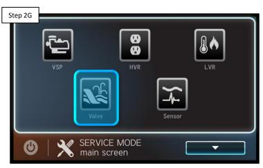
Put the controller in service mode and attempt to force the valve on. IF the still does not rotate, replace the Hub PCB (HLXHIOPCB). IF the valve rotates, go to 2H.
