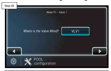
Make sure valve actuator is programmed to the correct port. To confirm, also test the actuator on the other port. IF programming is confirmed, go to step 2C. IF not, program the valve using quick edit.
