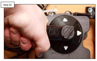
Verify the actuator shaft is engaged (as shown above). IF the valve moves freely, when rotating the handle, pull up on the handle to engage, IF engaged, proceed to step 2D.
