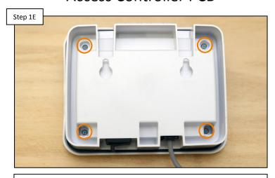
On the back of the controller, remove the 4 screws that secure the controller display to the housing. This provides access to the controller PCB. Once complete, go to step 1F.
