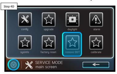
Follow steps to remove DDT (pg. 17). IF after programming is reestablished, the problem still persists go to step 4E. IF problem is corrected Backup configuration (pg. 14).
