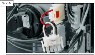
Verify selector plug matches incoming line power. IF it does not, power OFF & correct. IF OK, go to 1E.
