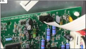
Verify ribbon cable is secure. IF cable is secure, replace display/bezel/keypad assy. (pg. 20) then go to 6D. IF NOT secured, reconnect. Check display for "CE"
