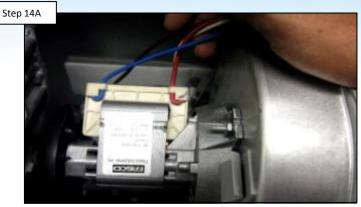
Check for bad blower and/or damaged blower vacuum switch wiring. IF OK, go to step 14B. IF damaged, replace compromised part (pg. 20).
