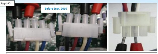
With power off, disconnect blower plug from ICB. <u>Models manufactured before Sept. 2010:</u> measure across pins 1-2 (black & red), then 3-4 (white & blue) for 8-9 ohms. <u>Models after Sept.</u> <u>2010:</u> measure for 4-5 ohms across the two terminal with wires. IF out-of-range, replace blower (pg. 20). IF correct, go to step 14E.
