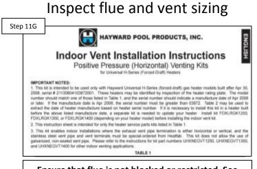
Ensure that flue is not blocked or restricted. See indoor vent sizing requirements in the heater's Installation Manual/Indoor Vent Instructions. IF OK, go to step 11H. IF NOT, contact installer.
