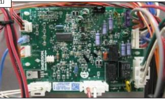
Inspect ICB wiring, ensuring all plugs are securely fastened. IF wiring is OK go to Step 1K. IF NOT, secure wiring/plugs then retest.
