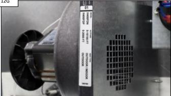
Check for damaged/wrong blower air inlet plate. IF wrong or damaged contact tech support (908) 355-7995. IF OK, go to step 12H. Verify correct flame sensor
