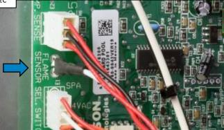
Ensure both flame sensor and gas valve are both securely fastened to the ICB. IF correct, proceed to step 12D.
