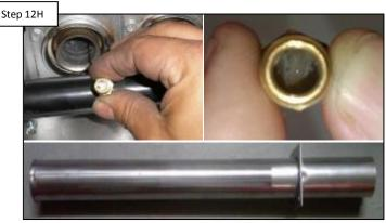
Inspect Gas Orifices & Burners for blockage. Clean as required. IF damaged, replace (pg. 20). IF NOT damaged, contact tech support (908) 355-7995.
