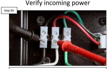
Ensure voltage is within 10% + or – of required voltage. IF voltage is correct, go to step 9B. IF NOT, then the problem is related to source power and must be corrected before error will clear. Inspect ground & neutral
