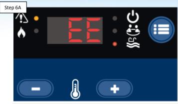
"EE" error indicates the you have a defective ICB board. IF this error appears, replace ICB (pg. 20). IF no EE error, go to 6B.
