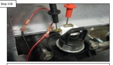
Remove wires from water pressure switch & measure continuity across terminals (while pump is running). IF open, replace water pressure switch. IF OK, go to Step 11C.
