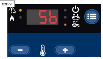
"Stuck Button" indicates display board is acting as if the button is being pressed and held. Replace display/bezel/key pad (pg. 20). Go to pg. 66 to test.
