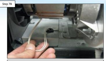
Power down and inspect ignitor wiring, ensuring ignitor plug is securely attached to the ICB. IF OK, go to step 7C. IF not, secure plug.
