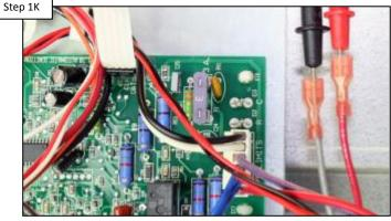
Disconnect and test the red and grey wires from the ICB. IF 22-28<u>VAC</u> is present go to step 1L. IF NOT, replace wire harness (pg. 20).
