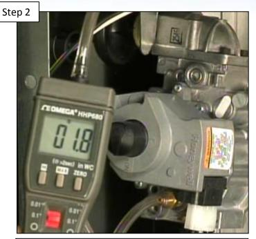
Manifold reading should be between 1.8"- 2.0" w.c for natural Gas or 6.8"- 7.0" w.c for propane.
