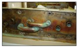
Sooted – Improper Fuel and Air Mixture.
