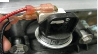
Inspect the water pressure switch wiring, ensuring wire harness terminals are securely fastened. IF damaged, replace wire harness (pg. 20). IF secure and free of damage, go to step 11B.
