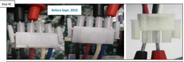
With power off, disconnect blower plug from ICB. <u>Models manufactured before Sept. 2010</u>: measure across pins 1-2 (black & red), then 3-4 (white & blue) for 8-9 ohms. <u>Models after Sept.</u> <u>2010</u>: measure for 4-5 ohms across the two terminal with wires. IF out-of-range, replace blower (pg. 20). IF correct, contact technical support (908)355-7995.
