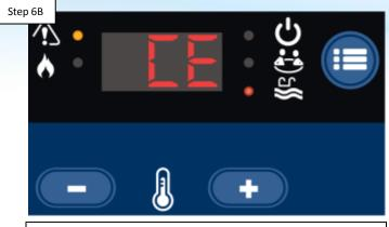
"CE" (communication error) indicates a problem between the ICB & display board. Cycle power OFF/ON. IF error persists, go to 6C.
