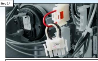
IF voltage selector plug matches voltage, go to step 2B. IF not, power down, replace FC1 & FC2 fuses, & switch plug to proper voltage.
