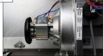
With the heater off (in "Stand By"), IF the blower continues to run/operate, replace the ICB. IF not, replace the blower vacuum switch (pg. 20).
