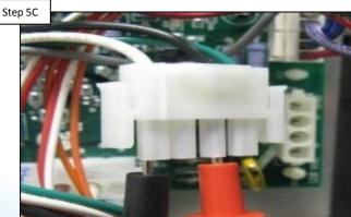
Disconnect the E10 connector from ICB. Verify 110-125<u>VAC</u> between 1-3 (white & black). IF present, replace ICB. IF NOT, replace wire harness (pg. 20).
