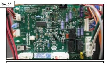
Inspect ICB wiring. IF wiring is damaged, replace the wire harness with a new wire harness kit (pg. 20). IF OK and the problem still exists, replace the ICB (pg. 20)
