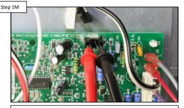
On the ICB, verify 22–28<u>VAC</u> between AC & COM terminals (pins 1 & 4). IF voltage is present, replace display/bezel/keypad. IF no voltage, replace ICB (pg. 20).
