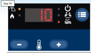
"IO" error stand for ignitor Open. IF this error appears, go to step 7B. IF "IO" does not appear, go to step 7D.
