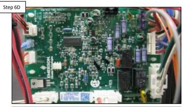
IF after replacing display/bezel/keypad, "CE" error persists, replace ICB (pg. 20). IF replacing ICB fails to solve problem, contact support (908) 355-7995.
