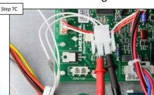
With power off, verify ignitor ohm resistance (8-25 ohms between 20°- 140°F). IF correct, replace ICB. IF out-of-range, replace ignitor (pg. 20).
