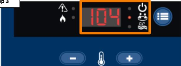
The 'SPA' indicator should illuminate & the display should show the Max Temp set point.
