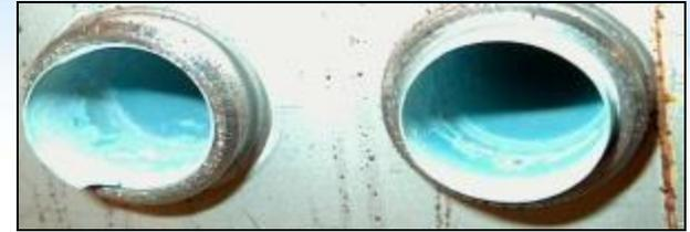
**Annealed Fins – Low Water Flow**
