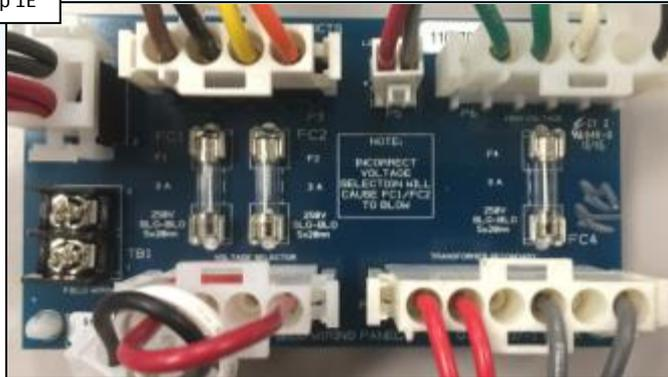
Inspect Fuse Board wiring, ensuring all plugs are securely fastened. IF correct, proceed to step 1F.
