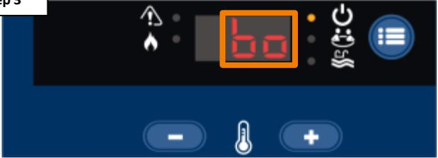
'bo' should appear on the display when the heater has successfully entered bypass mode.
