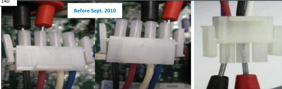
With power off, disconnect blower plug from ICB. Models manufactured before Sept. 2010: measure across pins 1-2 (black & red), then 3-4 (white & blue) for 8-9 ohms. Models after Sept. 2010: measure for 4-5 ohms across the two terminal with wires. IF out-of-range, replace blower (pg. 20). IF correct, go to step 14E.
