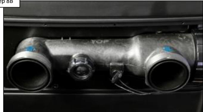
Verify the water inlet & outlet are not reversed; reversing these will often cause frequent occurrences of the “HS” error code. Follow the steps outlined in 8A. IF the thermistor checks-out, replace the ICB ([pg. 20](#)).
