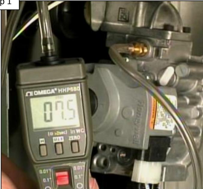
The static & load values should be within the levels listed on the data plate, example on [Page 17](#).
