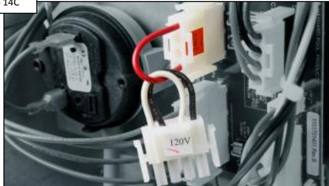
IF voltage selector plug matches voltage, go to step 14D. IF not, power down, replace FC1 & FC2 fuses (if open), & switch plug to proper voltage.
