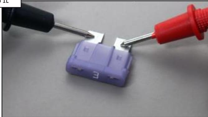
On the ICB, locate and test the 3A fuse for continuity. IF fuse is blown, replace it and go to [section 3](#). IF Ok, go to step 1M.
