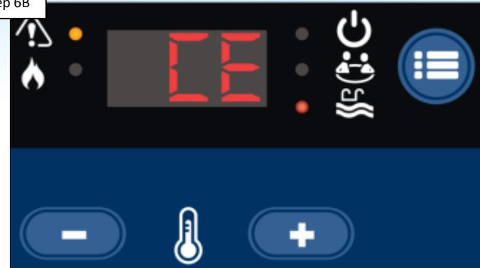
“CE” (communication error) indicates a problem between the ICB & display board. Cycle power OFF/ON. IF error persists, go to 6C.
