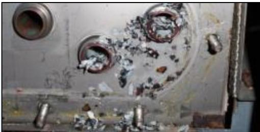
**Sooted – Improper Fuel and Air Mixture.**
