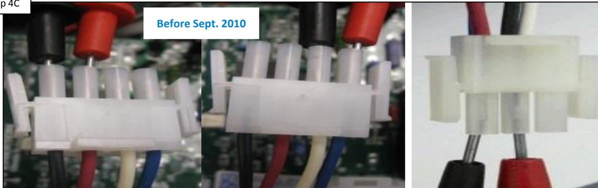
With power off, disconnect blower plug from ICB. Models manufactured before Sept. 2010: measure across pins 1-2 (black & red), then 3-4 (white & blue) for 8-9 ohms. Models after Sept. 2010: measure for 4-5 ohms across the two terminal with wires. IF out-of-range, replace blower (pg. 20). IF correct, contact technical support (908)355-7995.
