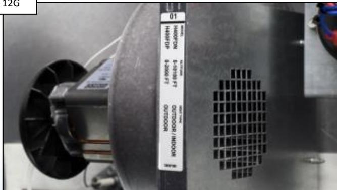
Check for damaged/wrong blower air inlet plate. IF wrong or damaged contact tech support (908) 355-7995. IF OK, go to step 12H.
