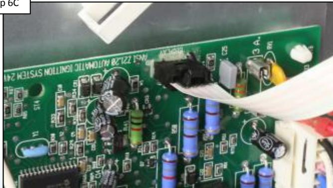
Verify ribbon cable is secure. IF cable is secure, replace display/bezel/keypad assy. (pg. 20) then go to 6D. IF NOT secured, reconnect.
