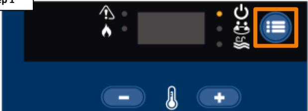
Press the 'MENU ICON' button to place the heater in 'STANDBY'.
