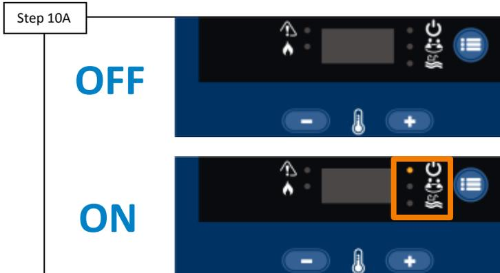
Power cycle the heater, in an attempt to clear an erroneous “HF” code. IF power cycling clears to the “HF” message and the heater fires, drop the temperature to suspend heating. IF “HF” reappears, go to step 10B.
