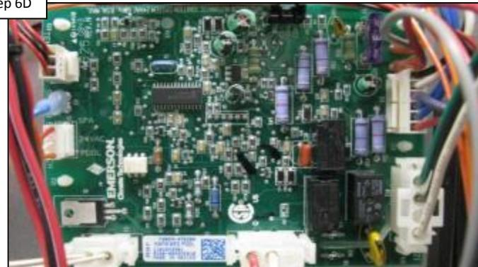
IF after replacing display/bezel/keypad, “CE” error persists, replace ICB (pg. 20). IF replacing ICB fails to solve problem, contact support (908) 355-7995.
