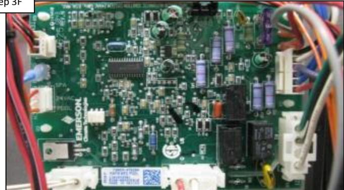
Inspect ICB wiring. IF wiring is damaged, replace the wire harness with a new wire harness kit (pg. 20). IF OK and the problem still exists, replace the ICB (pg. 20)
