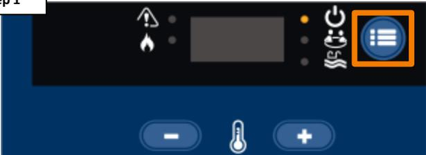
Press the 'MENU ICON' button to place the heater in 'STANDBY' mode.
