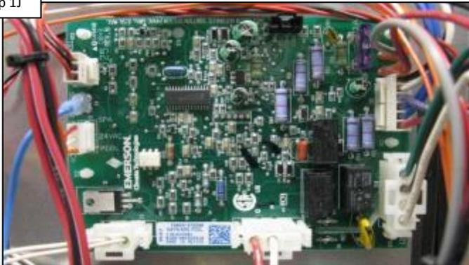
Inspect ICB wiring, ensuring all plugs are securely fastened. IF wiring is OK go to Step 1K. IF NOT, secure wiring/plugs then retest.
