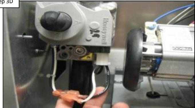
With power off, inspect the gas valve wiring for damage. IF damaged, replace the wire harness (pg. 20). IF OK, go to step 3E.
