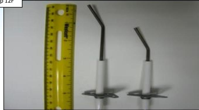
Verify that the installed flame sensor is 5". IF 3" is installed OR IF sensor is damaged, replace it with the 5" version (pg. 20). IF correct, go to step 12G.
