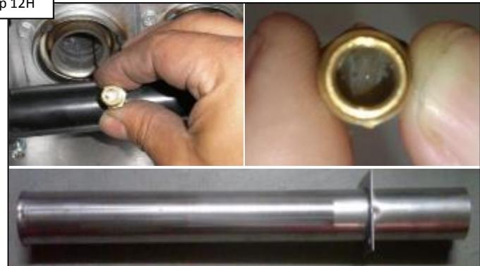
Inspect Gas Orifices & Burners for blockage. Clean as required. IF damaged, replace (pg. 20). IF NOT damaged, contact tech support (908) 355-7995.
