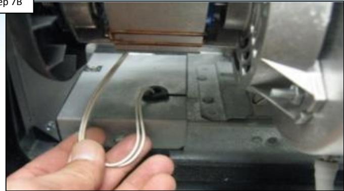
Power down and inspect ignitor wiring, ensuring ignitor plug is securely attached to the ICB. IF OK, go to step 7C. IF not, secure plug.
