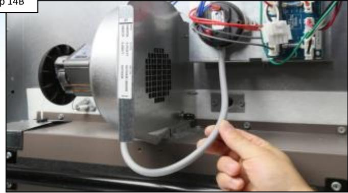
Check for damaged vacuum tubing as well as its connection to the blower. IF OK, go to 14C. IF NOT, replace vacuum tubing (pg. 20).
