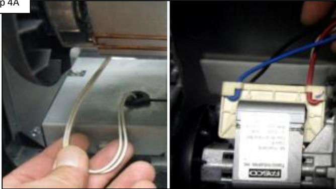
Inspect the Ignitor & Blower wiring. Verify insulation is not damaged. IF wires are damaged, replace the damaged part (pg. 20). IF OK, go to 4B.
