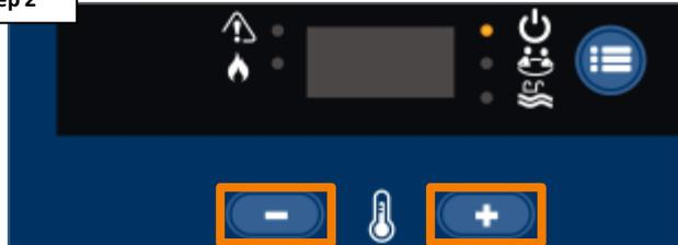
Press and hold the minus & plus buttons for 3 seconds.
