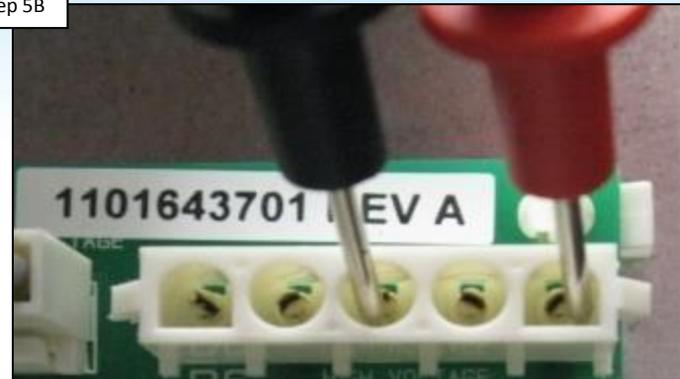
Disconnect the P6 connector and test voltage for 110-125VAC between pins 3-5. IF no/low voltage, go to step 5D. IF correct, go to 5C.
