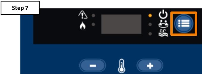
To finalize, press the 'MENU ICON' button until the heater goes back into 'STANDBY'.
