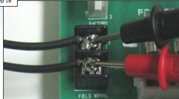
Verify 110-125 or 220-245V<sub>AC</sub> off fuse board (TB1). IF correct, go to 1D. IF NOT, correct source power.
