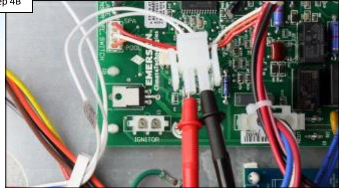
Disconnect ignitor from ICB & measure resistance of ignitor. Verify 8-25 ohms between 20°-140°F. IF correct, go to 4C. IF NOT, replace ignitor (pg. 20).
