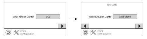
After naming the lights, select how many relays the lights are wired to. Note that the relays in this case are the "zones" on the Smart Power Transformer. If you would like the lights to always run together, then select multiple zones. If you would like then to run individually, then select only one.
