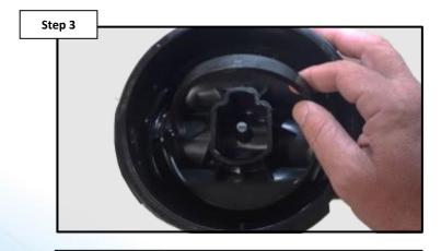
Using handle, lift hub assembly out of the body.
