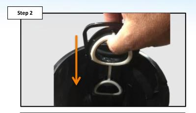
Lubricate inward facing seals with silicon lube and install seal carriers by firmly pressing them down into their slots.
