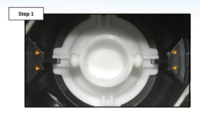
Install waste port seal carrier by aligning the locating features (arrows) on the carrier and the bottom of the valve body
