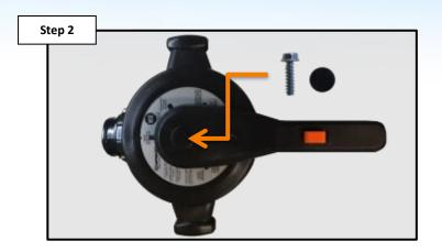
Insert the screw into handle & tighten with a 3/8" socket & ratchet. Align and press handle plug into slot to cover screw.
