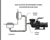
are individually rated for 515 GPM. For a desired flow of 130 GPM, a minimum pipe size from **Chart 1** is selected at 3". At the desired flow of 130 GPM one cover could be partially blocked and the total suction outlet flow would be below the rated 515 GPM of the remaining suction outlet. Since there are two outlets flowing in normal operation, and the allowable velocity in the branch piping is only 3ft/sec with both outlets flowing, the branch piping would require 3" pipe size.
