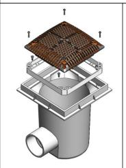
Installation Notes for WG1061HF2PAK2: When properly installed, the sump lip will be about 3/16" below finished surface of the pool. The finished surface of the pool should be flush to the top of the mud shield.
