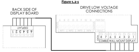
Connection wire must be rated for a minimum of 300V, and may be up to 500 feet in length. Use removable 6-position terminal block connectors for wiring connection to display and motor drive board taking care to note the wire colors and corresponding numbers next to the connectors. Do **not** connect to the upper input terminals shown as light gray above.
