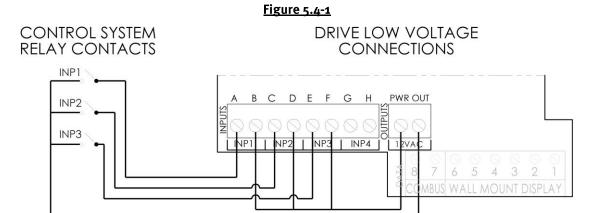
Connection wire must be rated for a minimum of 300V. See section 6.6.11 for more details. Do **not** connect to the lower "COMBUS" or wall mount "DISPLAY" data terminals.
