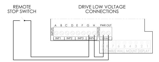
Connection wire must be rated for a minimum of 300V. Switch must be latching type; pump is stopped when circuit is closed.
