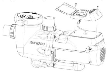
Figure 4.13-2: Adding the Blank Cover
