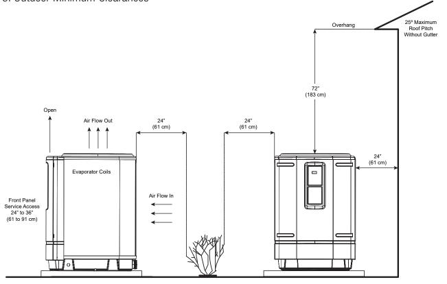
NOTE: The clearances shown above are for best practice and we encourage the use of the best practice clearances when the space is available. Exceptions can be made where the size of the lot or the configuration of fences, walls or other associated structures do not allow for the best practice clearances. Testing has shown our heat pumps can be installed as close as 12" (coil sides) from a restriction (Wall, fence, etc.).
