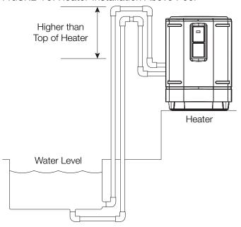
FIGURE 11: Typical Plumbing to Pool
