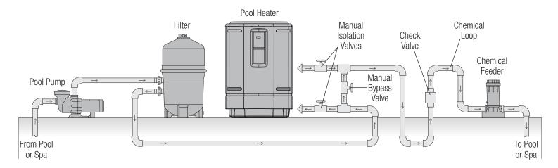
**CAUTION:** Improperly adjusted manual bypass valves will result in damage to the heater if the flow rates are not maintained under all operating conditions as specified in listed SPECIFICATION.
