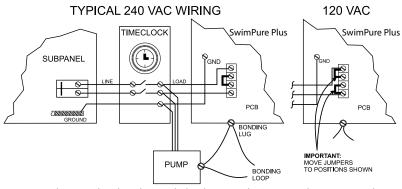
Note: Wire the pump directly to the timeclock -- do not use the Swimpure Plus as a junction box.
