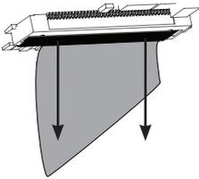
Use a fingernail or suitable tool to unlock the lever (shown in black). Gently pull the lever open in the direction of the arrows shown. When the lever unlocks, the ribbon cable will slide out of the connector.
