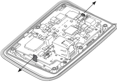
Flex retaining clips outward and gently pull up on the circuit board.
