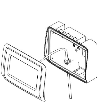
Remove 4 screws and separate the face from the Control Pad housing.
