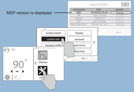
Before connecting the Wireless Terminal to the OmniLogic system, verify that you have the latest OmniLogic MSP firmware version. The firmware version displayed in "System Info" should be the same as the latest version available for download on the web. Follow the screens above to locate your MSP firmware version and go to Step 3 to find the latest firmware version on the web.
