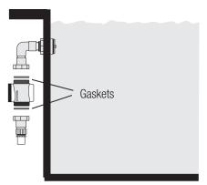
Using the supplied gaskets, attach the Cell Vessel to the Elbow Assembly and Hose Pipe Assembly. Do not tighten.
