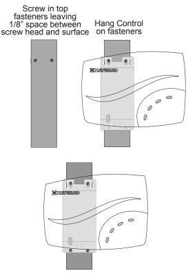
Screw in bottom fasteners securely.
