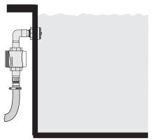
With the Hose Clamp already on the flexible pipe, slip the pipe on to the Hose Pipe Assembly as shown. Tighten the Hose Clamp firmly.
