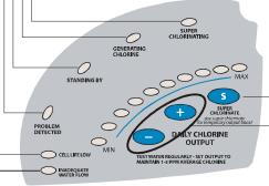
Illuminates when there is no flow or low flow through the Cell. The pool filter pump could be in its "off" cycle. If this is not the case, refer to the Troubleshooting section in this manual.
