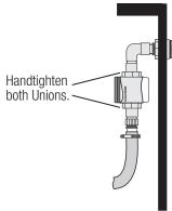
6. Position the Vessel in a manner where the Cell can be easily inserted and removed. Secure the Vessel by handtightening both Unions.
