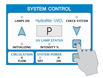
While the "P" is displayed, push the Enter key on the keypad. The HydroRite will go into normal operation and the UV lamp status (Intensity %) will be shown in the display. The HydroRite should remain powered at all times; the UV bulbs will go on and off with the pool filter pump.
