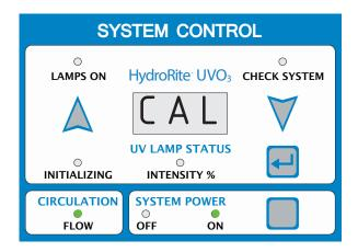
During calibration, the HydroRite LED display will cycle back and forth between "CAL" and the amount of time remaining to complete calibration. At the end of the calibration period, the HydroRite will either display a "P" for pass or "F" for fail (refer to Troubleshooting for failed calibration).
