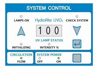
The Intensity will start out at approximately 100% and will slowly decline over time. When the UV lamp status reaches 70%, an internal alarm will be displayed and will require that the HydroRite be cleaned. Refer to Maintenance section for cleaning information. After cleaning, the HydroRite should return a higher Intensity value and continue normal operation. Over time, additional cleanings may be required and eventual bulb replacement will be necessary.
