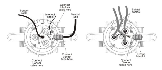
Venturi Booster Pump Wiring
