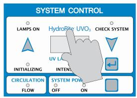
2) Access the Menu by holding the hidden button under the "Rite" in HydroRite.
