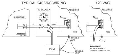
Note: Wire the pump directly to the timeclock -- do not use the AquaRite as a junction box.
