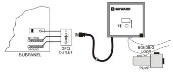
**Bonding:** A lug used for bonding is attached to the bottom of the AquaRite enclosure (see diagram below). The AquaRite must be bonded with an 8 AWG copper wire (6 AWG Canada) to the pool bonding system.
