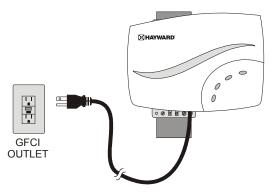
After being powered on for the first time, the Salt & Swim 3C will run a diagnostic routine which can take up to 30 seconds. During this time, various LEDs will turn on and off. When finished, the Salt & Swim 3C will display a blinking INADEQUATE WATER FLOW LED and a solid STANDING BY LED. Keep the Salt & Swim 3C powered for the remainder of this procedure and go to Step 3.
