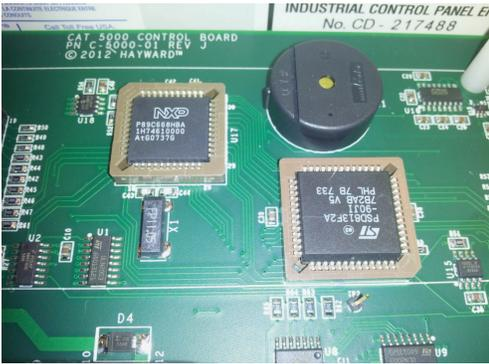
9) Press chips into sockets with same text orientation as old ones.
