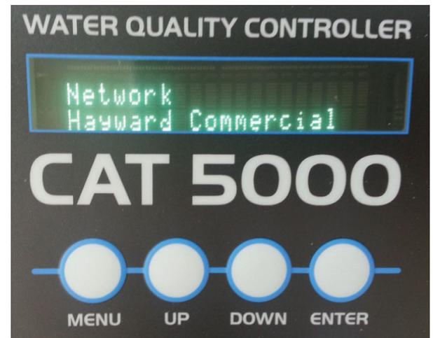
5) Scroll down to find your wireless network. Press ENTER to select. If display shows "None", then please allow an additional 5 minutes for unit to try to find networks.
