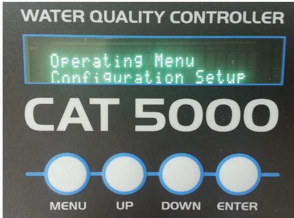
2) Plug in controller and wait at least 5 minutes after powering up. Press MENU. Scroll up to "Configuration Setup" and press ENTER.
