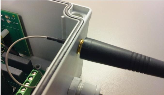
21) Hand-tighten the rubber antenna in place. (Note that washer and nut will remain visible).
