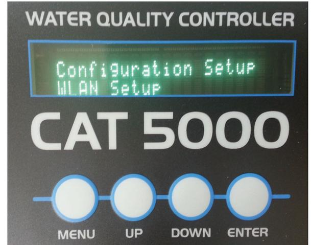
3) Scroll up to "WLAN Setup" and press ENTER.
