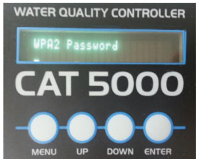
9) Using the UP and DOWN buttons, input the password to your router, then press ENTER. Allow at least 5 minutes for unit to establish network connection, depending on your wireless network speed.
