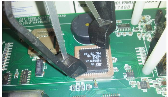
6) NOTE: BEFORE PULLING BOTH CHIPS, NOTE TEXT ORIENTATION ON EACH CHIP. (One chip shown removed). Using the chip puller supplied, remove old processor chips. (These must also be return-shipped to Hayward in supplied anti-static case).
