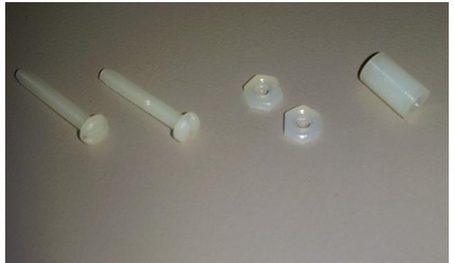
12) Gather nylon screws, nuts and spacer for fastening transceiver to motherboard.
