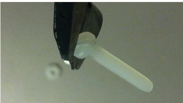
13) On ONE screw only, cut off one edge of screw head as shown. This prevents interference with antenna cable socket when assembled.
