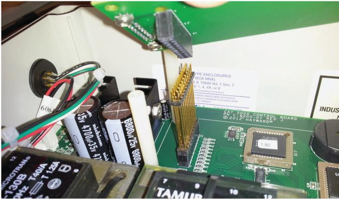
3) Remove board completely from unit by wiggling and pulling straight up.
