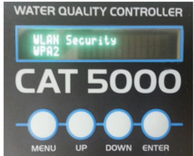
7) Select relevant security setting. Security setting types are as follows, and can be found on your router or by contacting your internet service provider.\*
