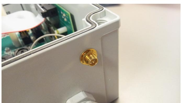
20) Install lock washer and nut and tighten with pliers.
