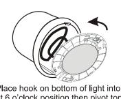
Place hook on bottom of light into niche at 6 o'clock position then pivot top of light into niche.
