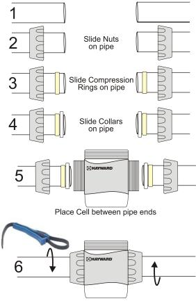
Insert pipe into Cell. hand tighten Nuts, and then use the included strap wrench to tighten an additional 1/4 turn
