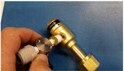
When done attaching the regulator to the solenoid valve, the assembly should look like the image below. Be sure to snug both fittings that fasten to the regulator.
