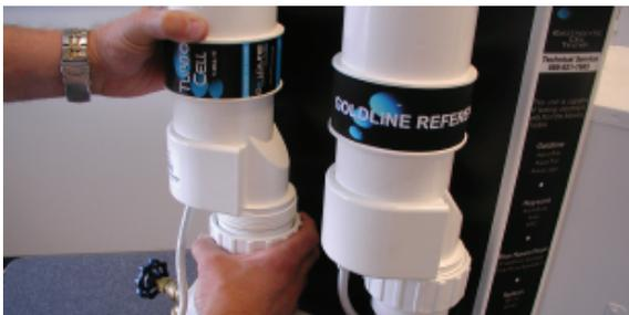
Install the customer's cell in the cell tester. Hand tighten the cell union (no tools) and make sure that the drain valve is closed. Do not attempt to test a cell with visible deposits.
