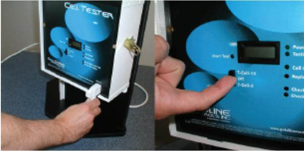
Plug the customer's cell into the control using the designated cell connector. Determine which model you are testing, T-CELL-15 or T-CELL-5. This information should be found on the customer's cell label. If there is any question as to which model you are testing, call technical support at (908)-355-7995. After determining the model, perform the following:
