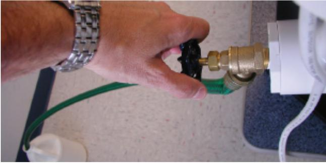
With a hose connected to the drain valve, remove all of the salt solution after the test is complete. Note that the solution is now heavily chlorinated and should be handled with care. Discard the solution by following the instructions below.
