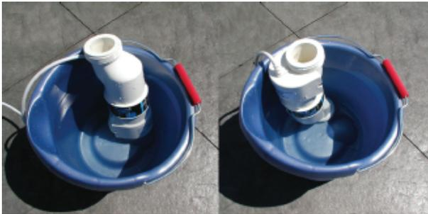
Using gloves and proper eyewear, prepare a solution of 2 parts water, 1 part muriatic acid in a suitable cleaning container by adding 2.5" of acid to 5" of water. **NOTE: ALWAYS ADD ACID TO WATER; NEVER ADD WATER TO ACID.**
