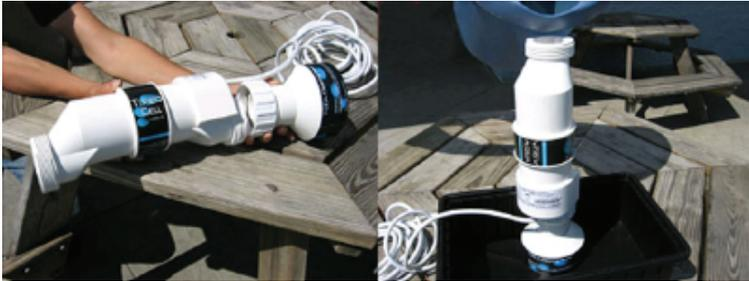
Using gloves and proper eyewear, prepare a solution of 2 parts water, 1 part muriatic acid in a suitable container. Mix enough solution to fill the inside of the cell (~1.5 qts). **NOTE: ALWAYS ADD ACID TO WATER; NEVER ADD WATER TO ACID.**
