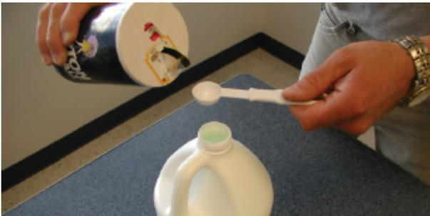
In a 1 gallon jug, add 2 teaspoons (use the included spoon) of non-iodized table salt to 1 gallon of room temperature tap water. Shake well. This procedure should yield a concentration of ~3200ppm.
