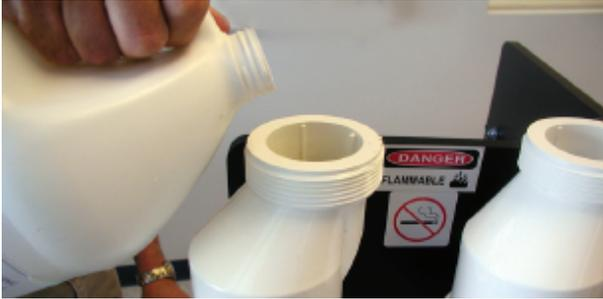
Pour the salt solution into the customer's cell until the level rises to within  $\frac{1}{2}$ " of the top of BOTH cells. This will ensure that the solution completely covers the fins inside of the cells.
