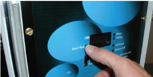
Push the "Start Test" button on the control. The test will take roughly 70 seconds. When the test is finished, the "Replace Cell" or "Cell Good" LED will light.
